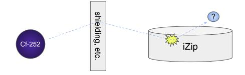
Though we started with neutrons out of Cf-252, we find that it's mostly secondary photons that ultimately deposit energy in the IZIPs.
