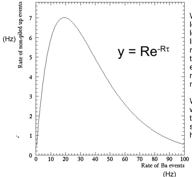
We will read out 52ms trace lengths (needed for filtering low-frequency noise). This limits usable total interaction rate to 7Hz per detector, due to pulse overlap. Piled-up events will have different noise properties and so are not useful!
