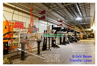
Fermilab staff have been busy getting the Main Injector and Recycler ready for beam. This photo shows the area of the tunnel where the MI8 beamline splits into the Main Injector and Recycler injection lines. *Photo: Marty Murphy, AD*
