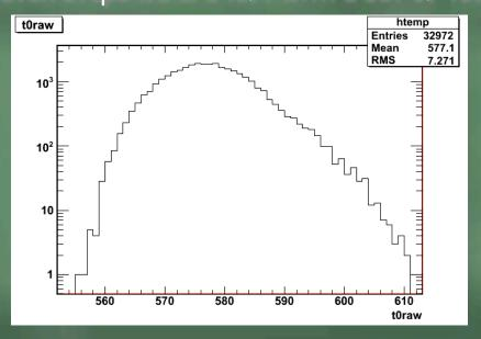
The values range from 560 ns to 590 ns for prompt particles with RMS ~0.8 ns due to energy slewing, the vertex t0 variation, etc.
