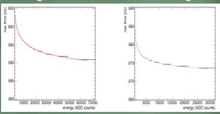
The Functional Form of the slewing correction from calibration table as a function of energy sum of the PMTs of an example tower in the CEM and PEM with the data
